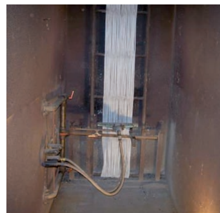
Fig. 8: Cable flame propagation test according to IEC 60332-3 cat. C
